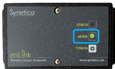
Blinking Green LED - Device Successfully Joined
